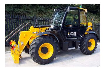
Max lift capacity **3,500kg**Max lift height **9,500mm**Max forward reach **6,520mm**Capacity at maximum reach **500kg**Engine power gross **75hp(55kW)**
